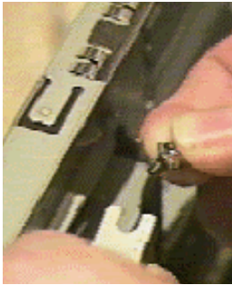
Figure 2-9. Removing the bracket screw
